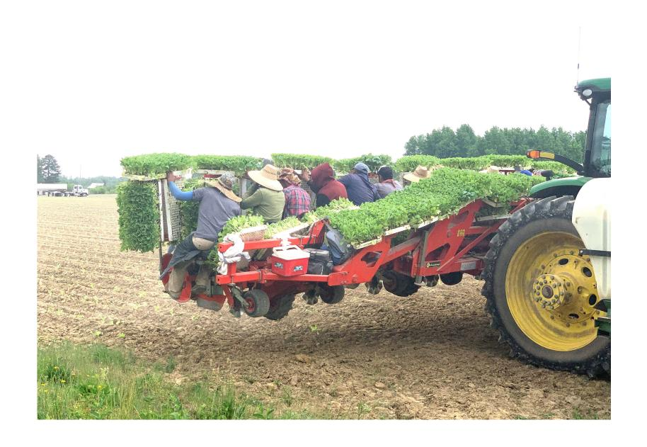
These workers in Nash County are planting (setting) tobacco. They ride in the back of the tractor, pulling seedlings from trays that have been loaded from nearby nurseries. The machinery pulls each seedling from its hand-loaded mechanical transplanter and plants it in the ground.
